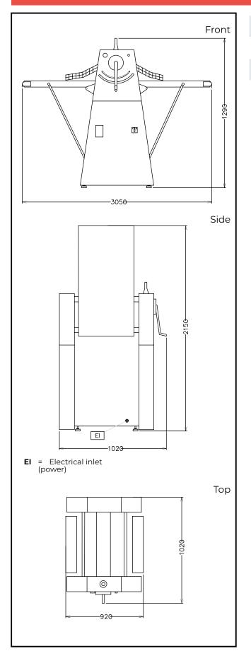
Electric Supply voltage: 400 V/3 ph/50 Hz **Total Watts:** 1.1 kW Key Information: External dimensions, Width: 3050 mm External dimensions, Depth: 1020 mm External dimensions, Height: 1290 mm Net weight (kg): 240
